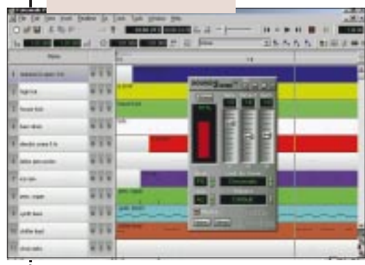
▼ FIG 4 SOUND 2 MIDI TAKES AN ANALOGUE SIGNAL FROM YOUR SOUND CARD'S EXTERNAL INPUT AND CONVERTS IT TO MIDI
